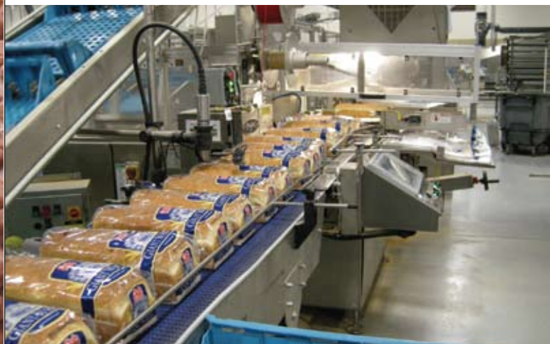
▲ Sliced, bagged, twist tied and date-coded bread is ready to be loaded into baskets coming from the basket washer.
